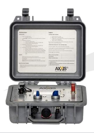
hard-wired together using AXXIS link sets. Up to 2 Blaster Boxes may be linked together on a single bench for a total combined firing capability of 1600 detonators per bench. When more than one separated bench is fired together it is possible to blast up to a total of 20 Blaster boxes with 16 000 detonators in total.
