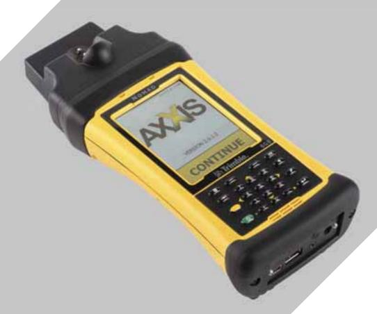
The AXXIS™Logger is a small, robust unit that is used to scan each detonator connector and allocate a delay period to that connector.
